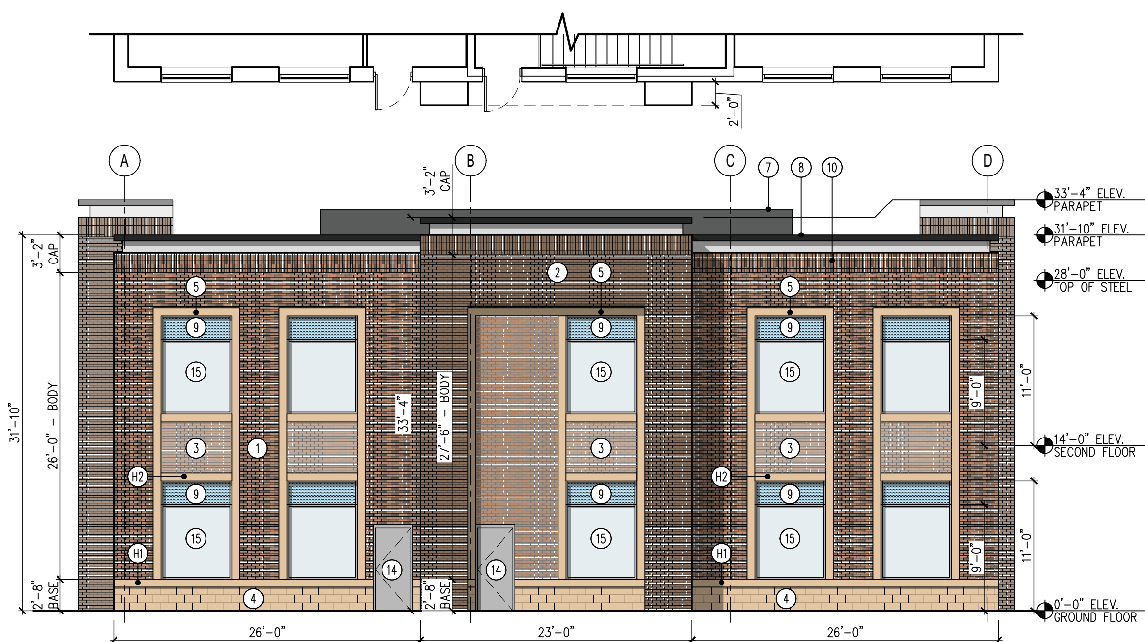
2 Building 1 Elevation West A201B SCALE: 1/8" = 1'-0"
