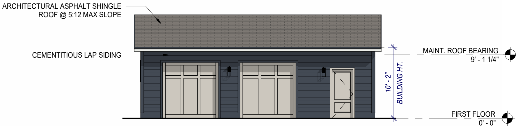
MAINTENANCE - NORTH ELEVATION-DP 3 1/8" = 1'-0"
