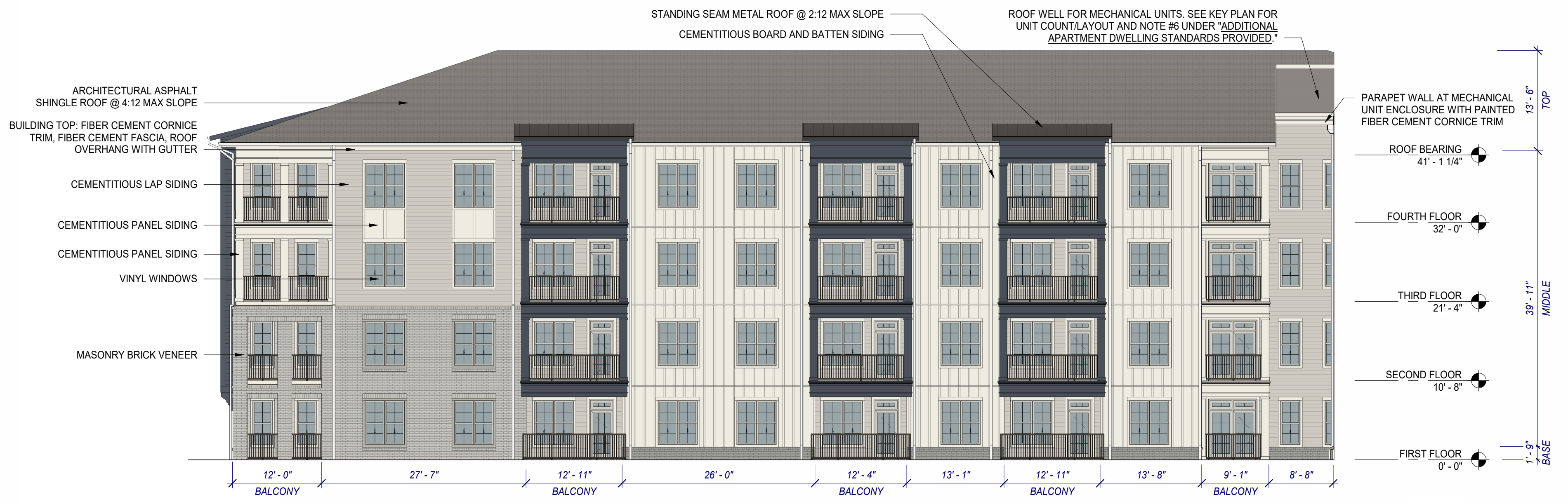
BLDG B COURTYARD - NORTH ELEVATION
