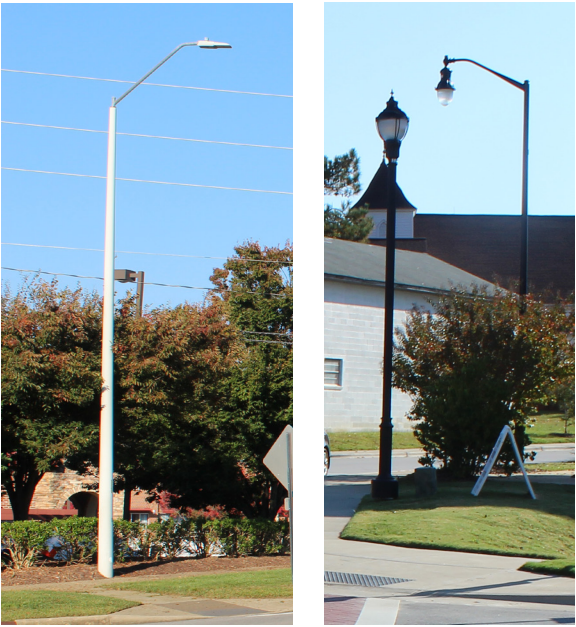
Examples of street and pedestrian lighting. Left, typical Duke Energy smooth fiberglass pole and LED Roadway fixture, to be used town-wide. Right, typical pedestrian and street light for Downtown Village District; pedestrian light is the Mitchell LED Top Hat with ribs, bands, and medallions with 16 ft mounting; post is a Decorative Aluminum Style VI; street light is a Teardrop LED on a Decorative Tapered Metal pole in black.
