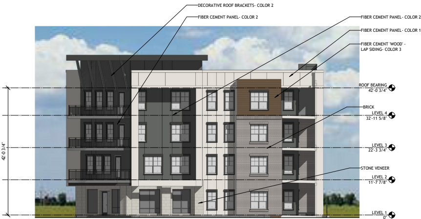
2 PRESENTATION ELEVATION - BLDG. 200 RIGHT- VIEW 4 A3-021 3/32" = 1'-0"
