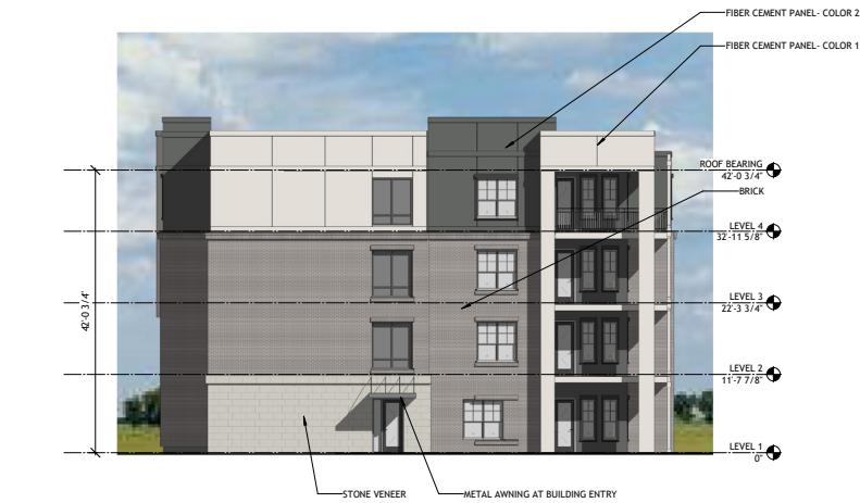
2 PRESENTATION ELEVATION - BLDG. 300 LEFT- VIEW 2 A3-030 3/32" = 1'-0"
