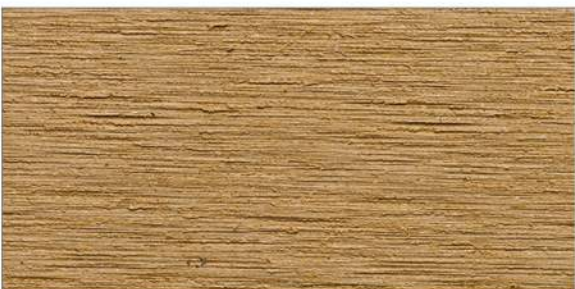
WPC-1: ALUMINUM/WOOD-PLASTIC COMPOSITE (TYPE 3 MATERIAL) TO MATCH GEOLAM 'TEAK' (WOOD PATTERN/COLOR)
